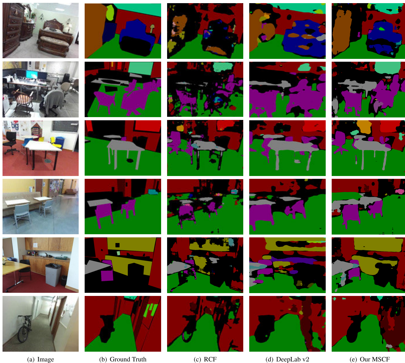
FIGURE 4. Qualitative results of our MSCF method compared to RCF and DeepLab v2 on SUN RGB-D. It can be seen that RCF pays too much attention to the details of the edges in objects, and thus is good at drawing the outline, such as tables, beds, and bicycles, but the black in the figure indicates that RCF fails to recognize the separated objects. On the contrary, DeepLab v2 can correctly recognize most of the segmented objects. But the segmentation effect is not as fine as RCF, since the edge of the segmented object tends to be blurred compared to RCF, as shown in (d). Due to the elaborate fusion of the strength from both RCF and DeepLab v2, our model outperforms DeepLab v2 in edge segmentation, and RCF in object recognition accuracy.
