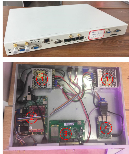
FIGURE 5. The automatic driving terminal designed by our laboratory, which combines INS, vehicle controller and Customer Premise Equipment (CPE). Internal structure: 1. Miniature transformer. 2. GPS module(In the actual test we replaced it with INS). 3. CPE. 4. Vehicle controller (Raspberry Pi 3).
