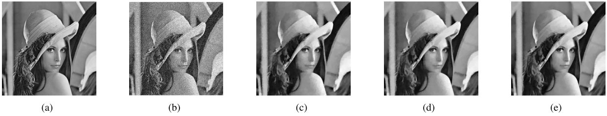
FIGURE 16. Obtained results on Lena; (a) True image; (b) Noisy image with \sigma = 22 ; (c) Resultant image by M3; (d) Resultant image by M4; (e) Resultant image by proposed method M2 ( c = 0.433, \lambda = 0.511 ).
