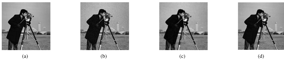
FIGURE 2. De-noised results on Cameraman; (a) Original image; (b) Noisy image with \sigma 1 = 15 ; (c) Resultant image by method M1; (d) Resultant image by method M2.
