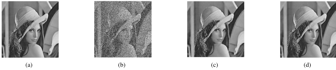
FIGURE 18. Restored results on Lena; (a) Original image; (b) Noisy image with salt and paper noise \sigma 2 = 50 ; (c) Reconstructed image by M5; (d) Reconstructed image by M2.
