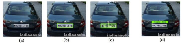
FIGURE 4. a) Original Image. b) Detected Image. c) Segmented Image. d) Recognized Image.
