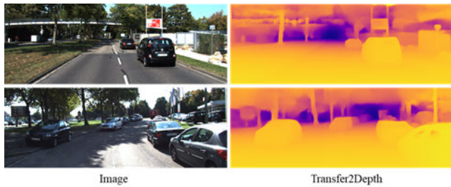
FIGURE 1. Estimated depth using Transfer2Depth. Input image and our estimated depth map on KITTI dataset.
