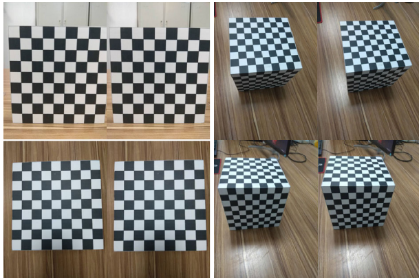
FIGURE 4. Checkerboard images for binocular camera calibration.
