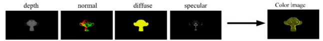
FIGURE 6. Color texture is generated from the other four images with the deferred shading technique.
