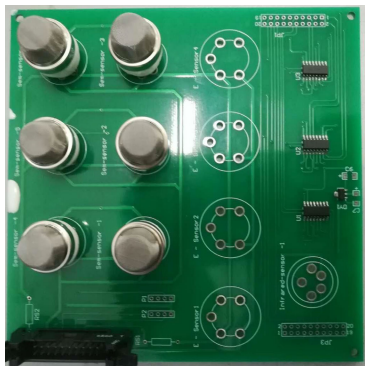
FIGURE 8. A photograph of the MQ-8 gas sensor array used in our experiments.
