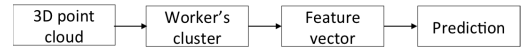
FIGURE 2. Prediction process from 3D point cloud data to prediction in the proposed method. Based on the 3D point cloud data, the method categorizes the point cloud and identifies 3D points representing a worker, as shown in Sec. III-B. We refer to the 3D points as a worker's cluster. The proposed method then computes a feature vector using the time-series data of the worker's clusters, as shown in Sec. III-C. Finally, the method predicts the reaching motion from the current time t to t + T by using a random forest, as shown in Sec. IV.
