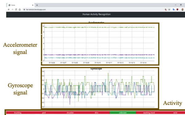
FIGURE 13. Web interface of the application with the activity bar in the bottom. The recognized activity is marked in green.
