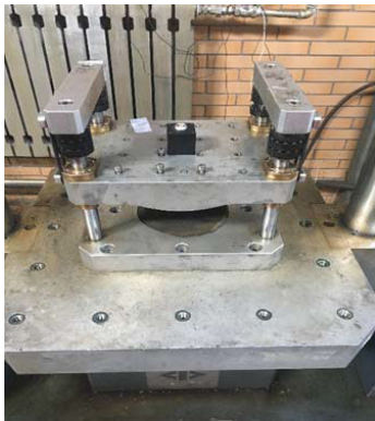
FIGURE 17. Double-layered plate-capacitor sensor.
