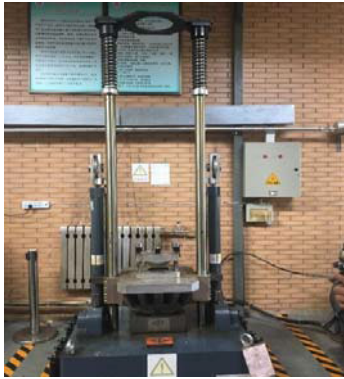
FIGURE 16. Hydraulic impact tester used in this study.
