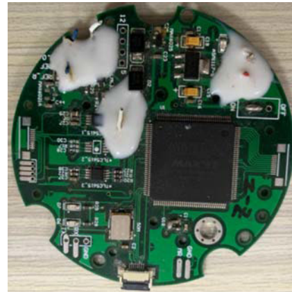
FIGURE 14. Front-side of the PCB for the sensor measurement circuit system.
