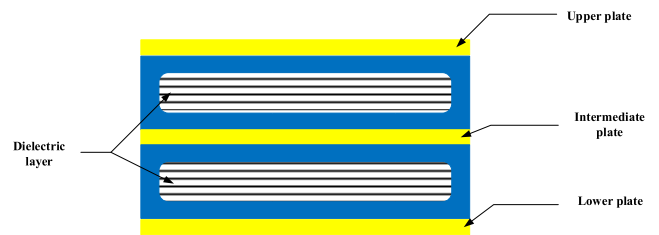
FIGURE 4. Schematic illustration of the capacitive sensor designed using a dielectric material.
