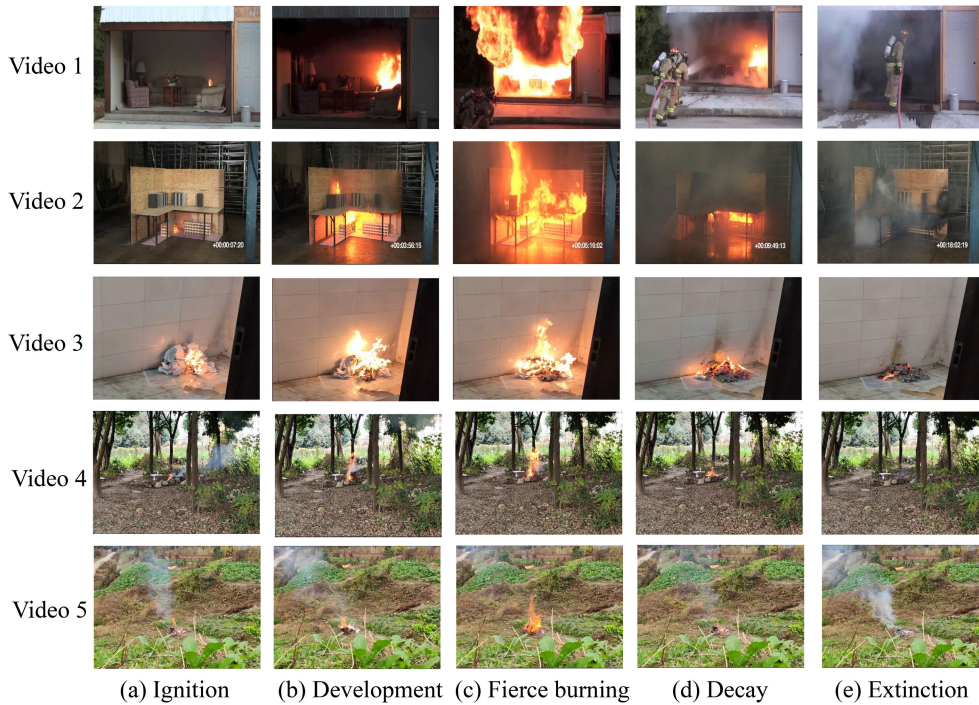
FIGURE 10. Examples of the whole evolution of a fire event. (a) Ignition. (b) Development. (c) Fierce burning. (d) Decay. (e) Extinction.
