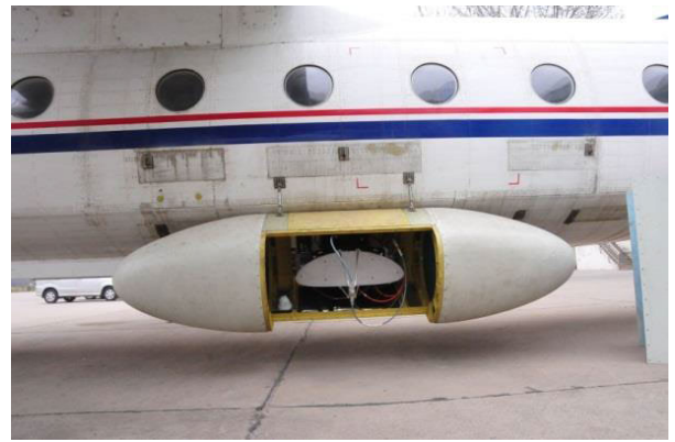
FIGURE 8. Airborne SAR antenna and its Servo control system mounted in the air pod.
