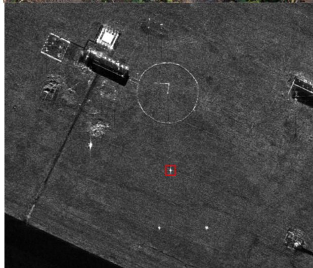
FIGURE 16. (Upper) triangular corner reflector and (lower) its corresponding SAR image in red square.
