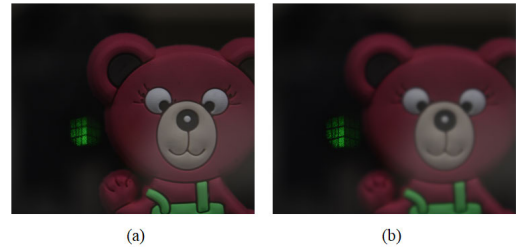
FIGURE 12. Results of holographic AR display when (a) the depths of the reconstructed image and the 'bear' are the same, and (b) the depth of the reconstructed image changes.
