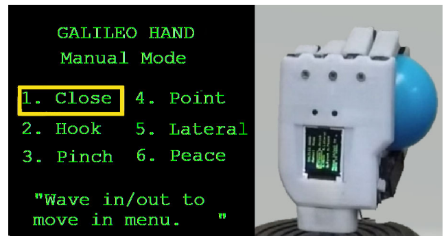
FIGURE 13. Graphical menu on the screen mounted on the prosthetic device (left) and the Galileo Hand performing a power grip on a ball (right).
