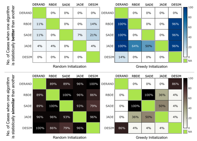
FIGURE 7. Statistical test to evaluate the performance of Differential Evolution classes. Wilcoxon tests were performed at the 5% significance level over 20 independent runs and overall robot trajectories. On top (bottom): the number of cases in which an algorithm in the row is statistically better (similar) than an algorithm in the column. In the left (right) side: situations using random (greedy) initialization.
