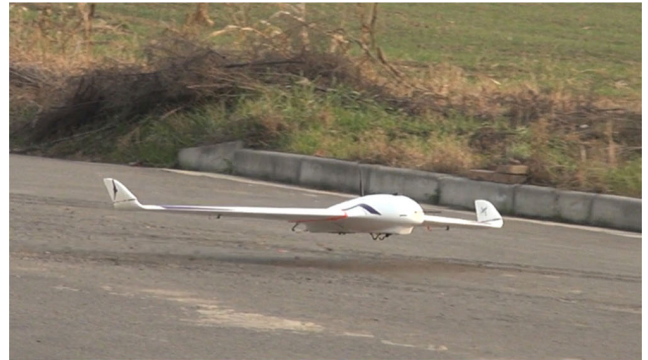
FIGURE 2. Fixed wing UAV with the Ellipse-N system.
