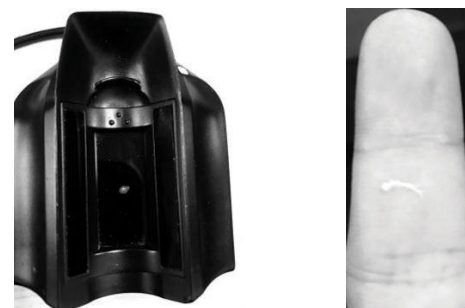
FIGURE 1. The conditions which will cause the loss of finger vein image information: polluted equipment mirror and peeling finger.
