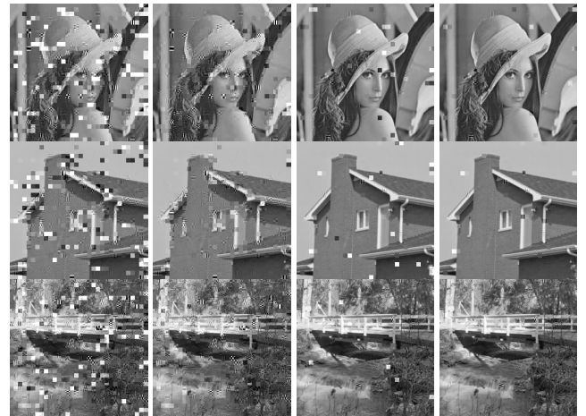
FIGURE 9. Test images Lena , House and Walkbridge recovered at SNR = 4 dB (STTC-ML), SNR = 4 dB (STTC-TV), SNR = 7 dB (STTC-ML), SNR = 7 dB (STTC-TV) (left to right) for JPEG coded image transmission.
