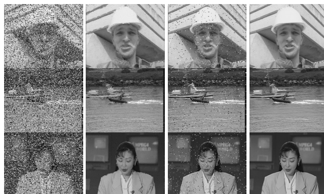
FIGURE 10. Reconstructed frame–53 of the test videos Foreman , Coastguard and Akiyo recovered at SNR = 0 dB (STTC-ML), SNR = 0 dB (STTC-TV), SNR = 4 dB (STTC-ML), SNR = 4 dB (STTC-TV) (left to right) for raw video transmission.
