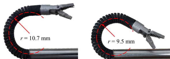
FIGURE 15. Bending condition of a flexible joint made of hard rubber.
