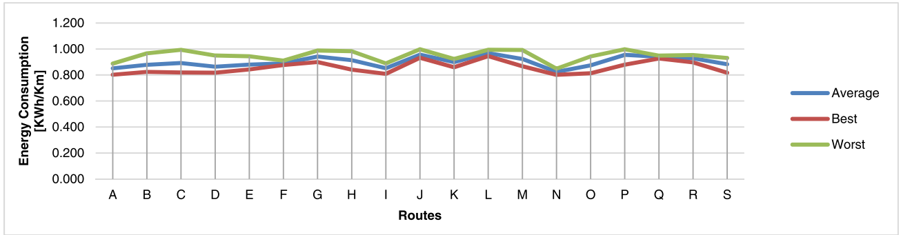
FIGURE 21. 100-days energy consumption over routes during peak hours (peak-1, peak-2, and peak-3).
