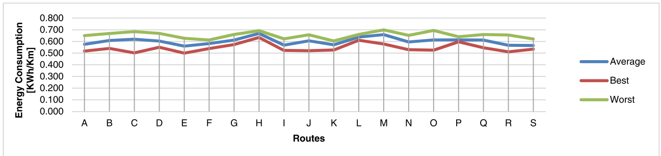
FIGURE 22. 365-days energy consumption over routes during normal hours (early morning, morning-2, afternoon and night).
