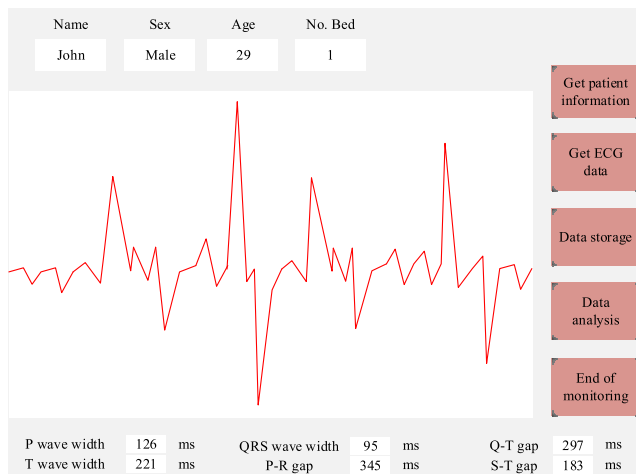
FIGURE 16. Remote server monitoring software ECG III leads waveform analysis.
