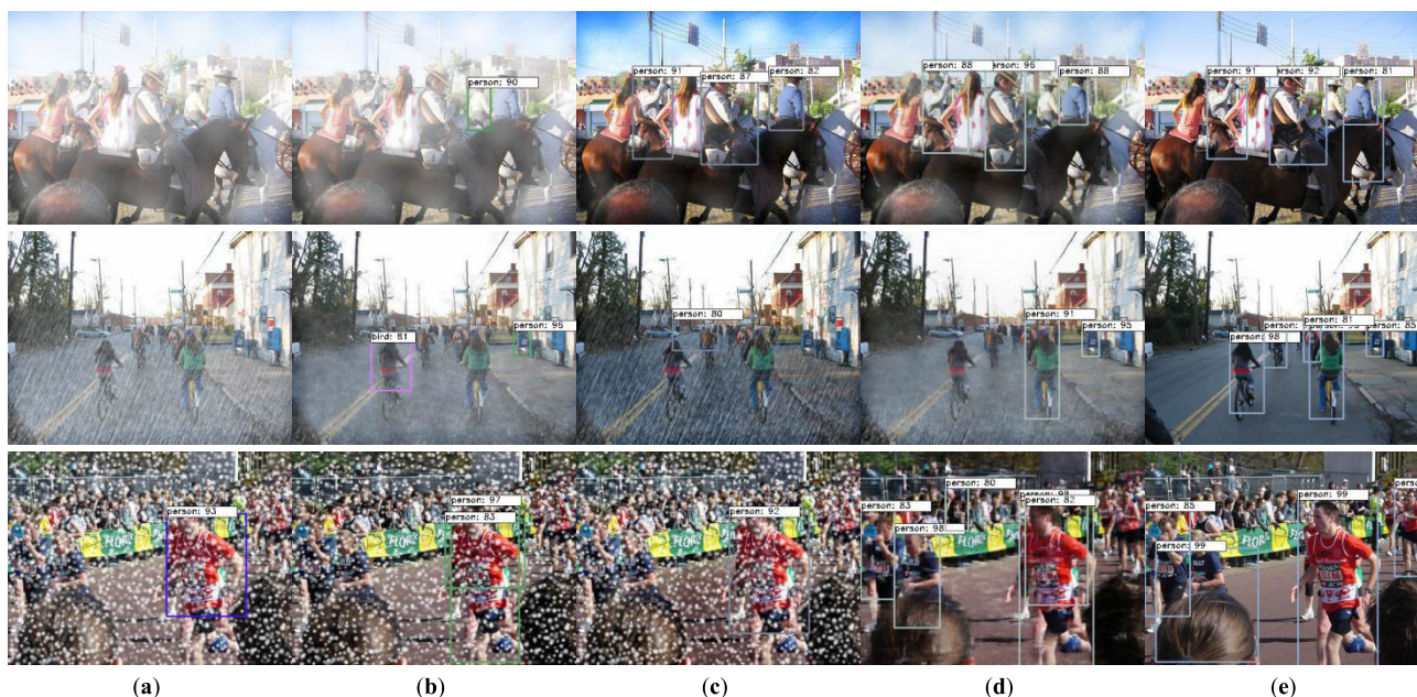
FIGURE 14. Samples of object detection (Faster-RCNN [54]) results after using clarity enhancement algorithms. From top to bottom, they are fog, rain streak and snowflake images. (a) Degraded images, (b) Processed by DDN [18], (c) Processed by DCP [8], (d) Processed by RASWNet, (e) Ground truth images.
