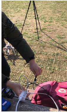
FIGURE 18. Detaching local base station during UAV flight and switching to NTRIP source.
