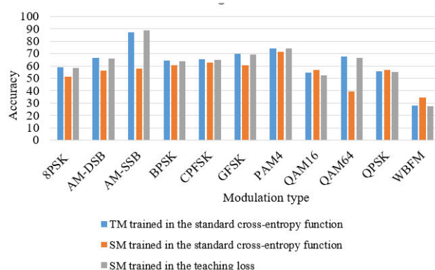
FIGURE 4. The accuracies of the proposed models in predicting for each class. The SM trained in the teaching loss shows a similar characteristic to that of the trained TM for different modulation types.
