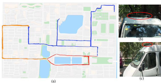
FIGURE 11. Outdoor evaluation, (a) figure of traces where we recording and testing our system around Tianjin University, tracks in red is under heavy traffic, with moving vehicle and amounts of random movement pedestrian; tracks in orange is under median traffic, with moving vehicle, little pedestrian; tracks in blue is under related static area, little moving vehicle and pedestrian. (b) front view of our system mounted on the top of van. (c) side view of the our system installed on the van, sensor is marked under red ellipse.
