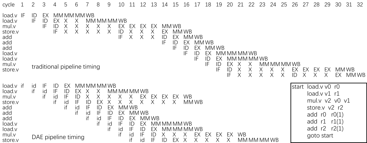
FIGURE 3. Pipeline timing of traditional RISC architecture and DAE architecture. (pipeline stages of FDU are in lower-case).
