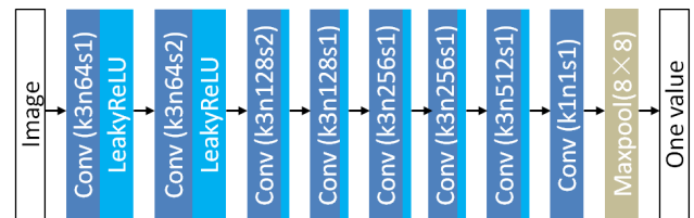
FIGURE 2. Architecture of our designed discriminative subnetwork. Each convolution layer is indicated with corresponding kernel size (k), number of feature maps (n), and stride (s).
