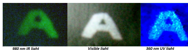
FIGURE 11. Images recorded through the designed optical device under infrared, visible and ultraviolet illuminations.
