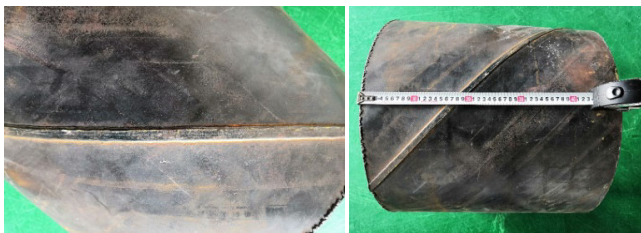
FIGURE 11. Actual outward appearance of spatial helical seam weld beads at steel pipe end.
