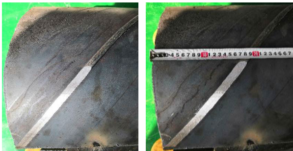
FIGURE 19. Robotic grinding result of helical seam weld beads at steel pipe end.
