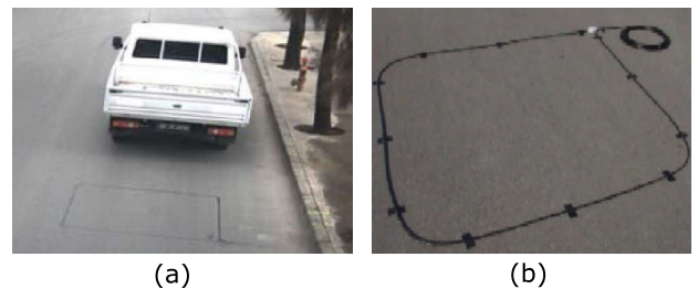
FIGURE 2. Types of loop detectors: (a) saw-cut loop [20]; (b) preformed loop [48].
