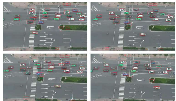
FIGURE 7. An example of an aerial image and vehicle detection using SVM [83].
