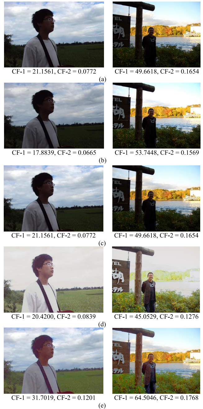
FIGURE 3. Restored Backlit Image. (a) Original image; (b) Yelmanov's model [23]; (c) Leow's model [24]; (d) Xin's model [20]; (e) the proposed optimal stretched image.
