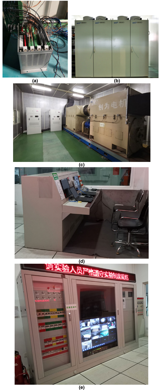
FIGURE 13. THE 3.6 MW POWER UNIT FULL TRUE WIND FIELD SIMULATION EXPERIMENT PLATFORM (a) The control box, (b) The power grid simulation platform, (c) The 3.6MW wind turbine unit experimental platform, (d) The operating floor, (e) The monitoring system.
