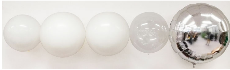
FIGURE 2. Evaluated balloons, from left to right: Qualatex untreated round 41 cm latex balloon, Qualatex untreated round 61 cm latex balloon, Qualatex round 61 cm latex balloon treated with UHF, Qualatex round 61 cm Bubble balloon and Qualatex round 91 cm Microfoil balloon.
