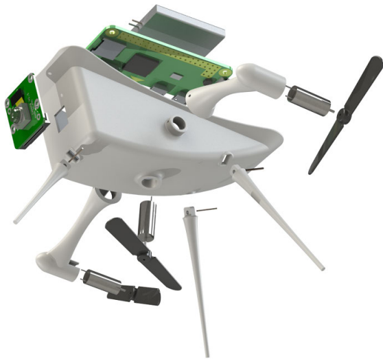
FIGURE 4. Exploded view of the robotic gondola. The electronics are depicted at the top of the figure, including the single cell Li-Ion battery. The camera is positioned in an angled configuration on the gondola and is depicted at the left of the figure. The modular rotor brackets and airship legs allow for easy replacement and fast modification.
