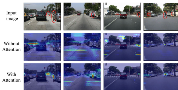
FIGURE 3. The visualization results on the test set of the Caltech dataset. We compare the visualization results with and without the use of dual attention network. The input images are from the test set of Caltech dataset. Pedestrians in the input image are marked with red circles.
