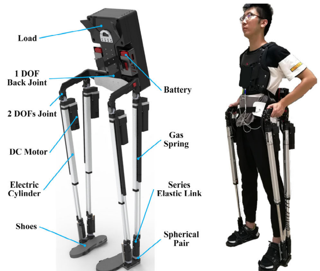
FIGURE 2. The composition of the exoskeleton mechanical system and the prototype with a wearer. PALExo can be mainly divided into three parts: the upper body, legs, and shoes. Each leg of the exoskeleton contains two active telescopic rods, which connect the upper body and the shoes through the hook and hinge at the end. The wearer in the picture is 188mm tall and weighs 79kg.
