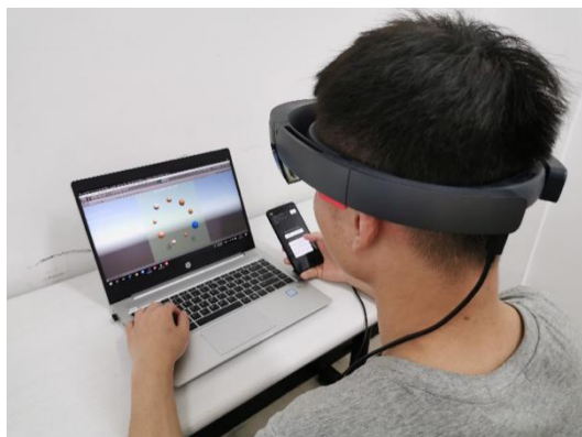
FIGURE 4. Experiment scenario where the subject wears the HoloLens while using a mobile phone to select the target.
