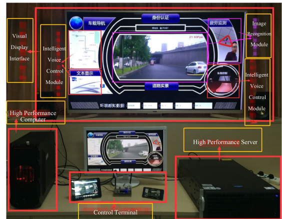
FIGURE 6. Human-car voice interaction and environment perception system.
