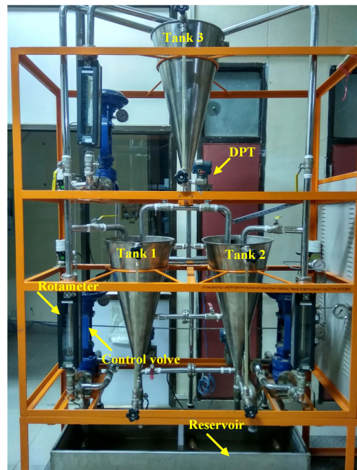
FIGURE 5. Real conical tank system used for identification.
