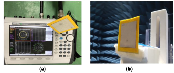
FIGURE 8. Antenna measurements for: (a) the reflection coefficient using a network analyzer, and (b) the radiation pattern in an anechoic chamber.
