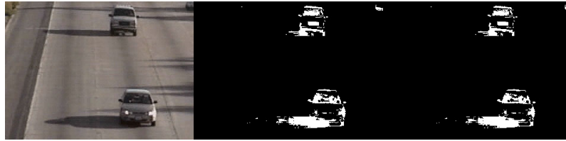
(a)input frame (b) H, S, V three-channel experimental result (c)S, V dual-channel experimental result
