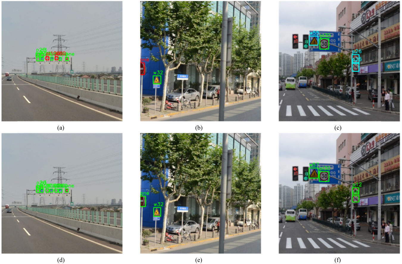
FIGURE 7. The upper row presents the experiment results of YOLOv3, and the lower row presents the detection results of YOLOv3 after performing data augmentation. The green box presents the correct prediction of the traffic signs, the red box represents the missed detections, and the blue box represents the false detections.
