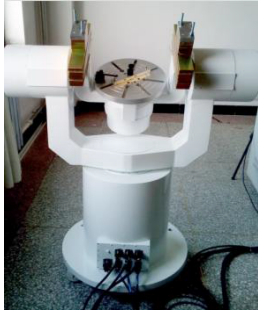
FIGURE 3. The three-axis LOS motion control device.
