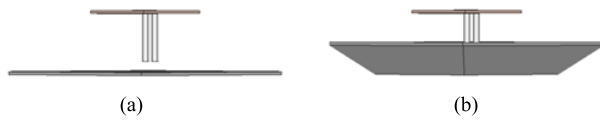
FIGURE 11. Two different shapes of the reflector. (a) square-shaped reflector. (b) cavity reflector.
