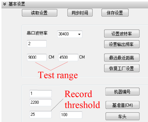
FIGURE 11. Setting the sensor parameters.
