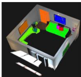
FIGURE 10. Generating 3D point cloud map with color annotation of object instance by experiment.
