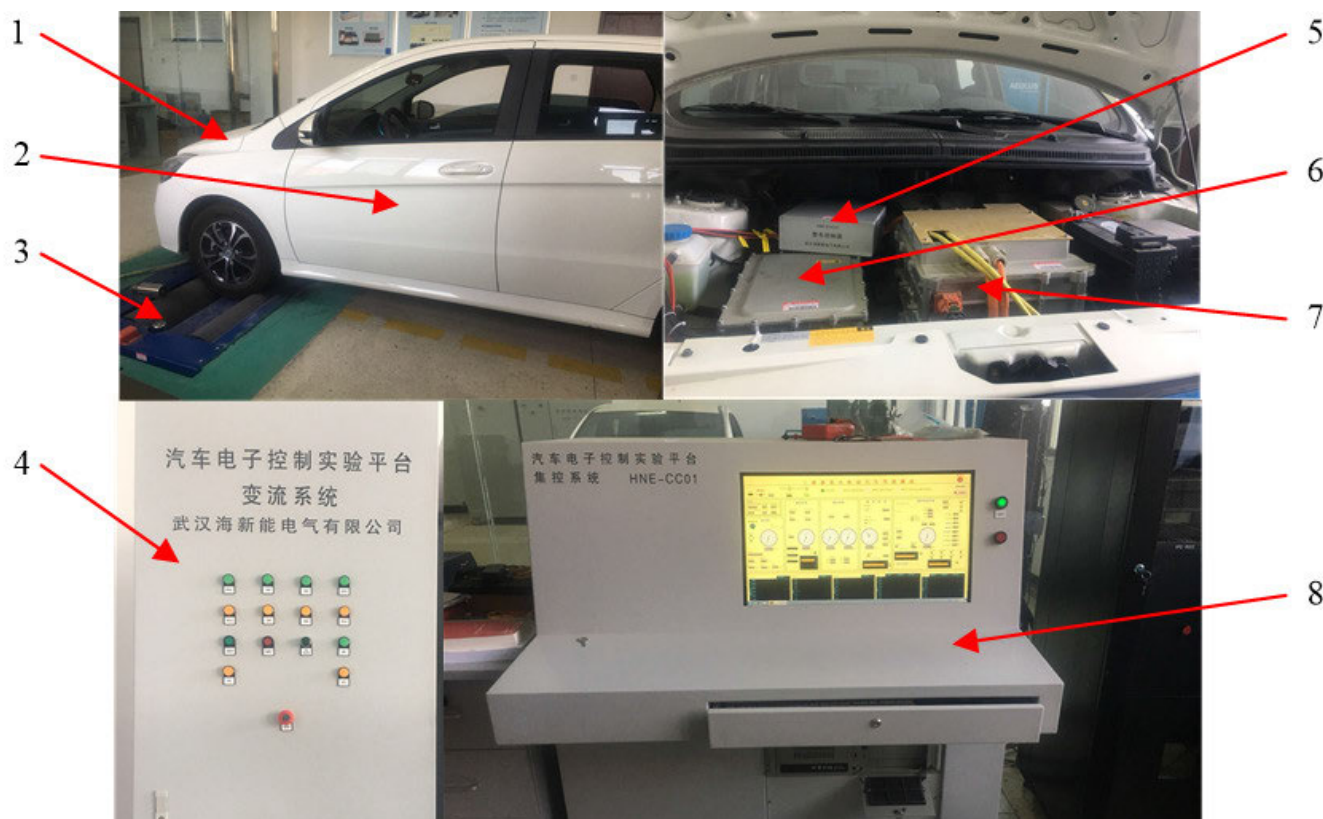
1. ICE and its controller; 2. Tested vehicle; 3. Dynamometer; 4. Inverter system; 5. Vehicle controller; 6. EM and its controller; 7. Battery and its controller; 8. Centralized control system.
