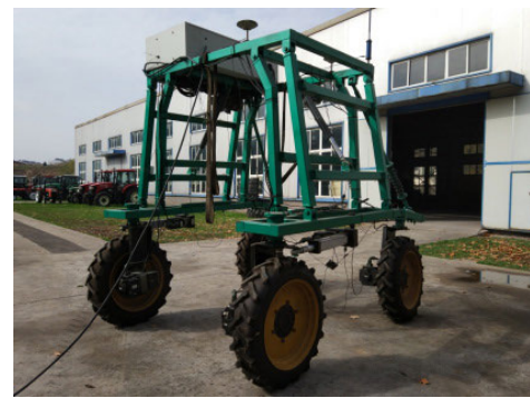
FIGURE 21. Experiment platform for the distributed electrically driven agricultural logistics.
