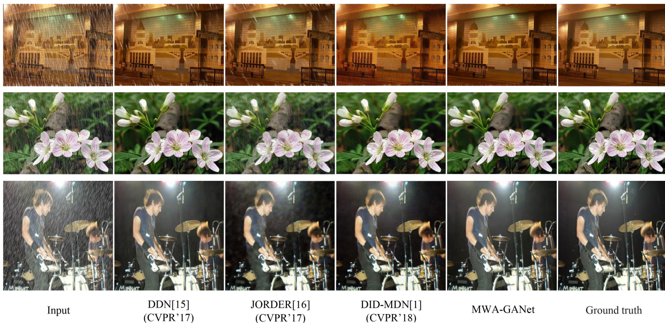
FIGURE 7. Rain-streak removal results on sample images from the synthetic datasets Test1 compared with other state-of-the-art single-image de-raining methods.
