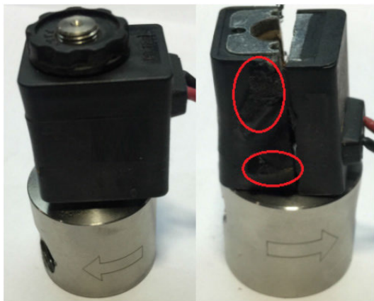
FIGURE 31. Comparison of a new SV and a failed SV.
